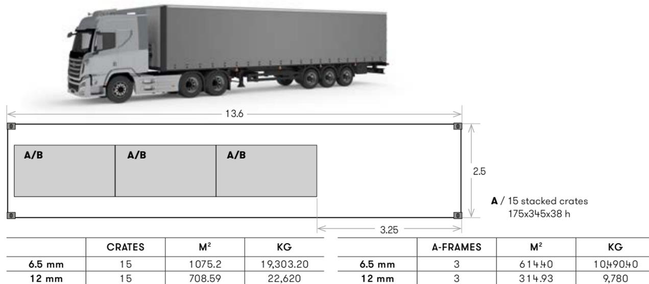
Take great care to balance the weights and check that the vehicle has sufficient payload for transporting all the weights loaded.
